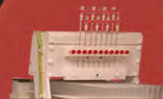
Dual filtration system with filter valve set, multi-sampling points with HPLC vial collection with same membrane filters
