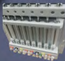
Syringe sampling system with accuracy to 1%
