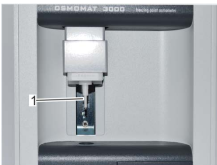
Fig. 46: Clean temperature sensor
