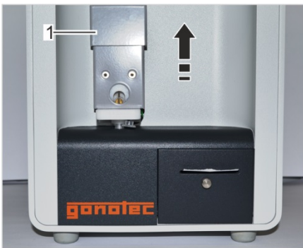
Fig. 130: Move elevator cover up
