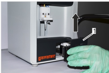
Fig. 134: Remove printer cover
