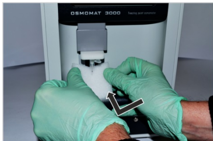
Fig. 20: Position transport safety device
