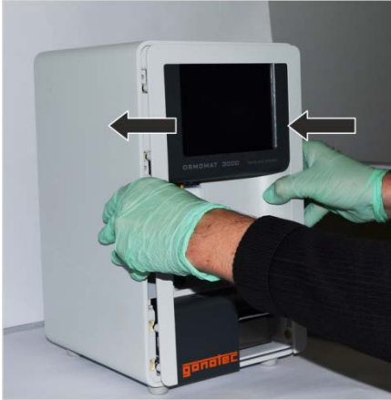
Fig. 137: Install device front panel
