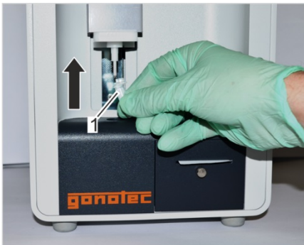
Fig. 94: Position measurement vessel
