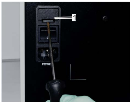
Fig. 112: Open microfuse cover
