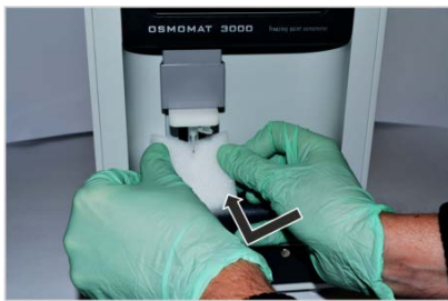
Fig. 149: Position transport safety device
