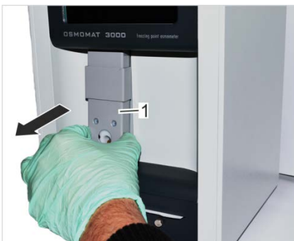
Fig. 132: Remove elevator cover
