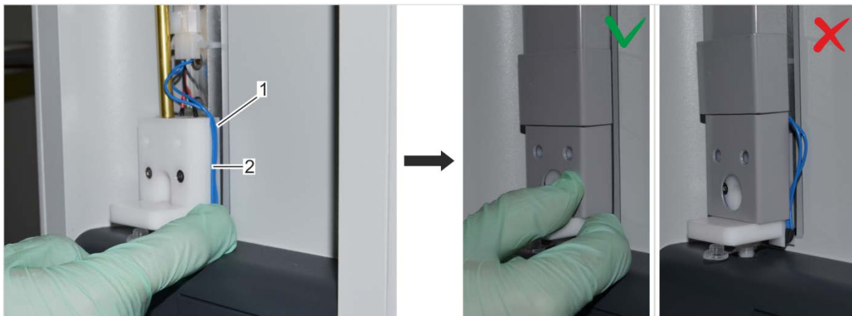
Fig. 138: Elevator cover with correct cable routing
