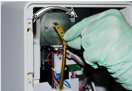
Fig. 92: Check free movement of cryst-needle
