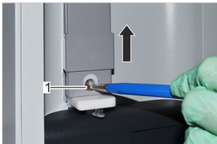
Fig. 110: Clean cooling nipple
