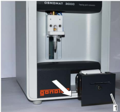
Fig. 133: Pull out printer
