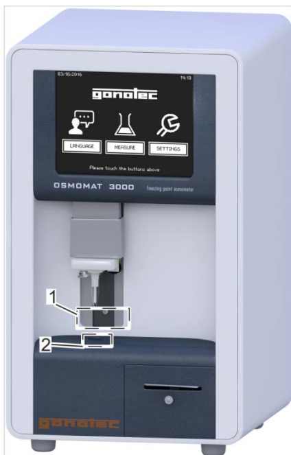
Fig. 142: Inspect device for foreign objects
