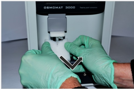
Fig. 25: Remove transport safety device
