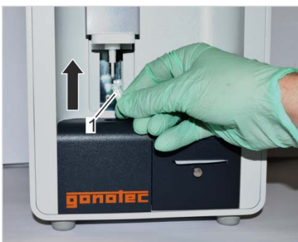
Fig. 70: Position measurement vessel
