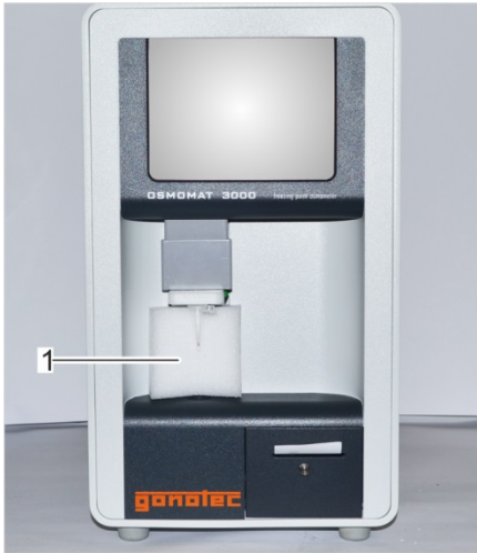
Fig. 24: Transport safety device
