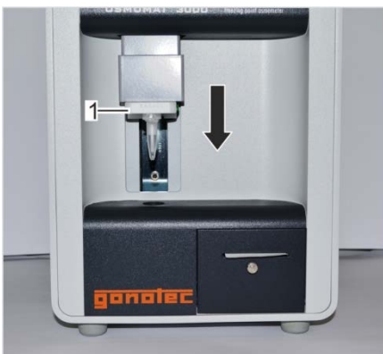
Fig. 54: Move elevator down
