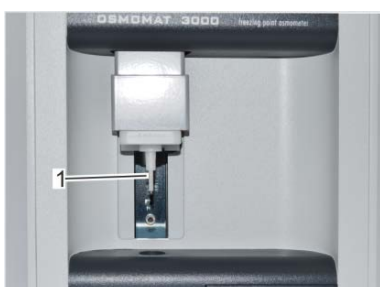
Fig. 57: Clean temperature sensor
