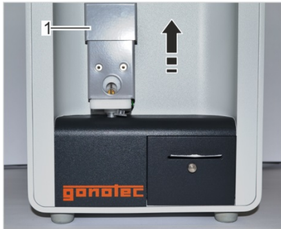
Fig. 96: Move elevator cover up
