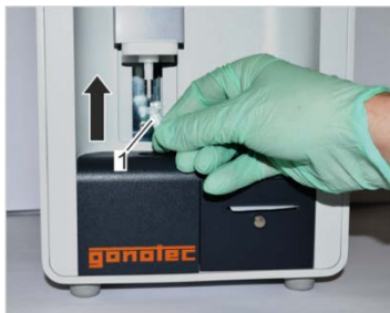
Fig. 82: Position measurement vessel
