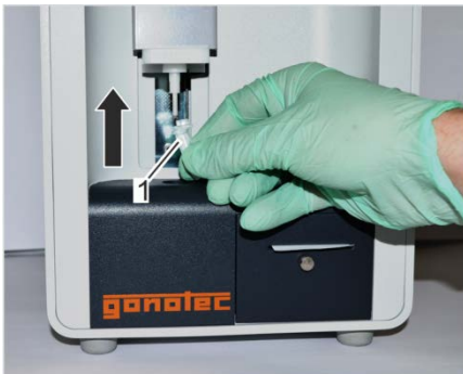
Fig. 64: Position measurement vessel
