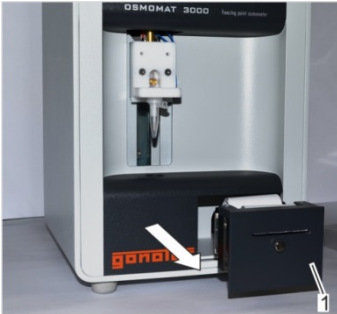
Fig. 26: Pull out printer
