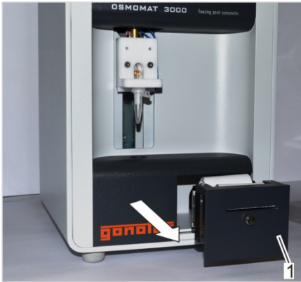
Fig. 117: Pull out printer
