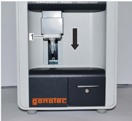
Fig. 71: Move elevator down
