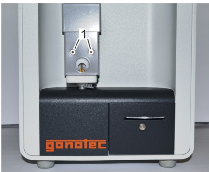
Fig. 131: Remove mounting screws
