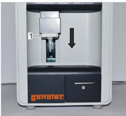
Fig. 76: Move elevator down
