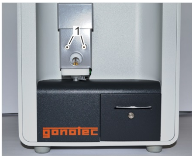
Fig. 97: Remove mounting screws
