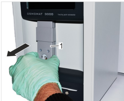
Fig. 98: Remove elevator cover
