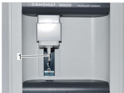
Fig. 66: Clean temperature sensor
