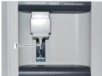
Fig. 56: Clean temperature sensor
