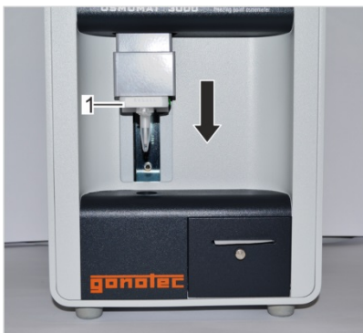
Fig. 95: Move elevator down
