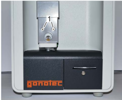
Fig. 139: Tighten mounting screws
