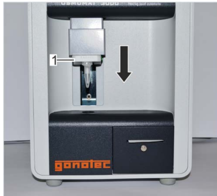
Fig. 65: Move elevator down
