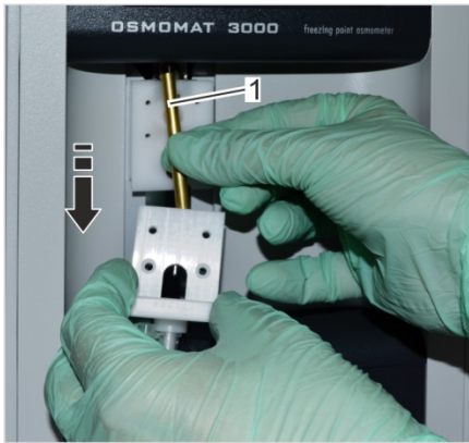
Fig. 101: Remove temperature sensor
