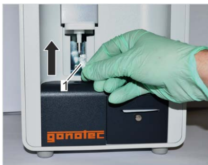
Fig. 146: Position measurement vessel
