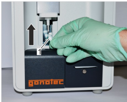
Fig. 19: Position measurement vessel
