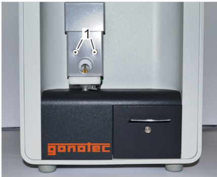
Fig. 109: Tighten mounting screws
