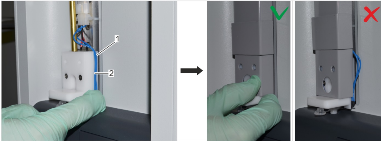
Fig. 108: Elevator cover with correct cable routing
