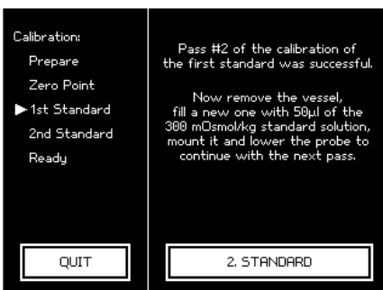
Fig. 77: Second calibration standard
